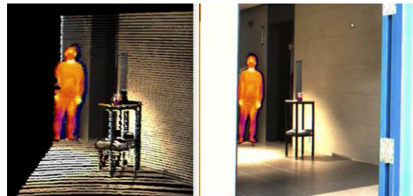
Figure 12. Fused Point Cloud with colour and thermal information and the corresponding colour image registered with the thermal image for detecting hot objects like a pedestrian and a tea cup.
