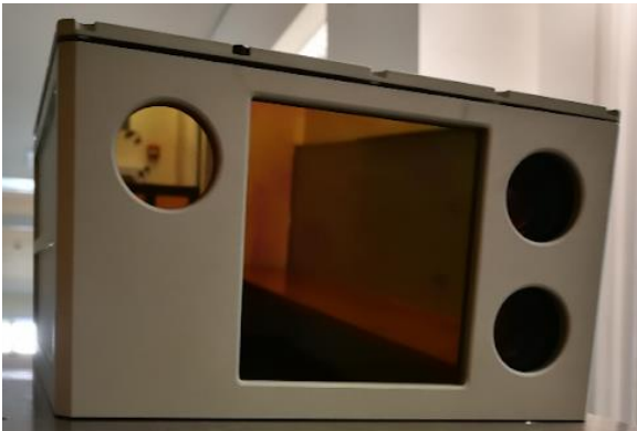
Figure 4. Multimodal fusion system based on LiDAR courtesy of Beamagine SL.
