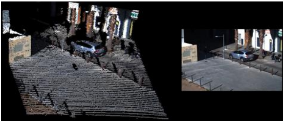
Figure 6. Fused Point Cloud with colour information up to 40 m range and its corresponding image.
