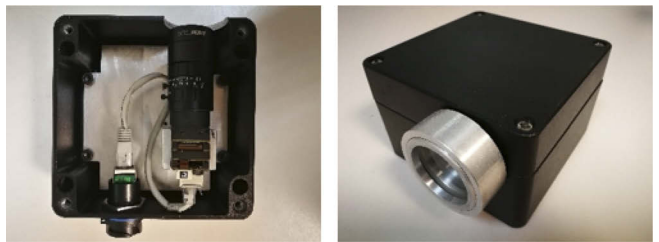
Fig. 3. Setup of the DOFP camera together with the QWP aligned with the horizontal axis (left) and enclosed camera within an IP68 cage to preserve the seal of the inner cavity (right).
