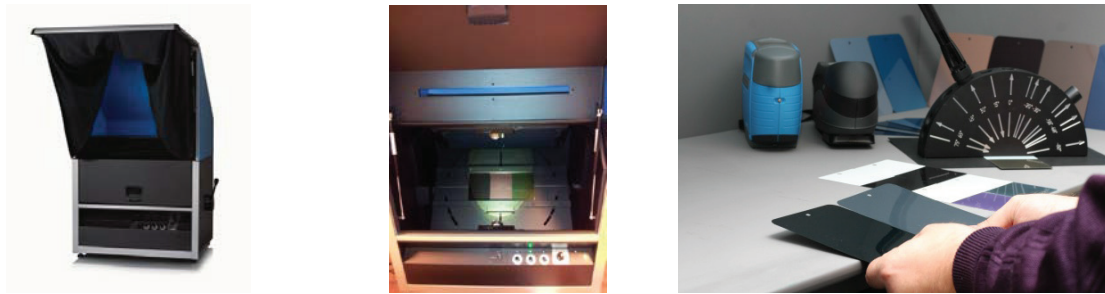
Figure 4 – Lighting booths analysed in this work. From to left to right: byko-spectra effect (exterior and interior view) and gonio-vision-box inside one Verivide CAC-150 cabinet (diffuse illumination), with some gonio-apparent panels and the instruments BYK-mac and X-Rite MA98
