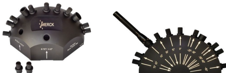
Figure 9 – Exterior view of the gonio-vision-box cabinet. Left: back side, showing some viewing directions in order to see some colour subgamuts of gonio-apparent panles in out-plane geometries. Right: front view, showing the wLED lamp at 45° incidence angle, and marking some viewing directions in order to simulate the measurement geometries of some multi-gonio-spectrophotometers (see Figure 2 and Table 1).
