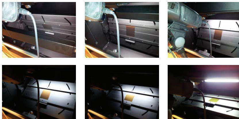
Figure 12 – Pictures of a typical gonio-apparent panel inside the byko-spectra cabinet such as it is measured by a PR-650 tele-spectroradiometer. Top, left to right: measurement geometries 45as110, 45as75 and 45as45. Bottom, left to right: 45as25, 45as15 and 45as-15.
