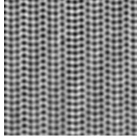
Figure 7.4.13 Confocal Image of a periodic structure of 0.4 micron period and 0.2 micron diameter.
