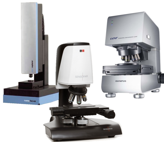
Figure 7.2.1 Some commercial Confocal instruments. Clockwise: nanofocus (disc scanning), Sensofar (Microdisplay Scanning) and Olympus (Laser Scanning).
