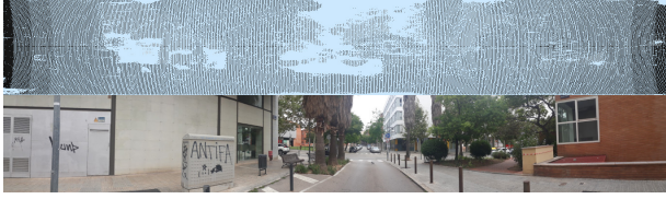
Fig. 2: Depth image obtained from the projection of the point cloud of a Beamagine LIDAR scan. Pixels without depth values are set to blue in the depth image to ease visualization. The photo below was taken some days after the captures from a similar point of view.
