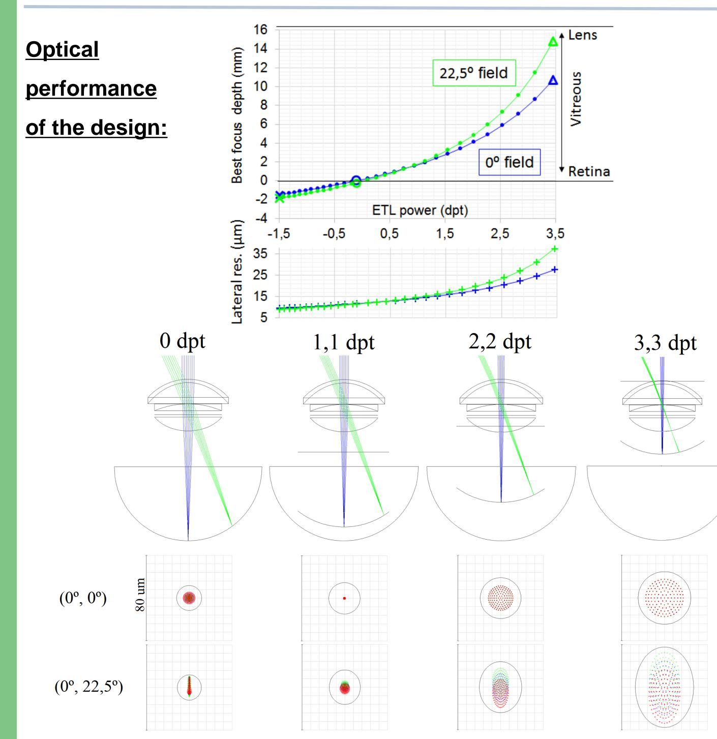
Focus tuning allows highlighting opacities at different depths of the
