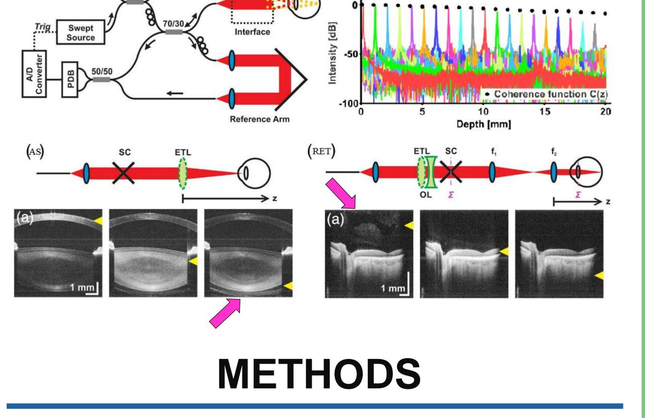
In this work we describe the design of a sample arm specially dedicated to vitreous imaging to be included in the long depth range SS-OCT instrument described in [2,3].
