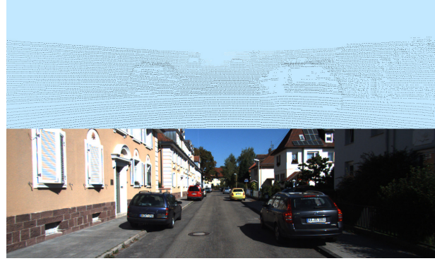
Fig. 1: Depth image obtained after the projection of a KITTI LIDAR scan, with its corresponding color image below. Pixels without depth values in the LIDAR scan are colored in blue in the depth image to ease visualization.
