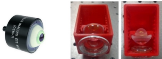
Fig. 4. (Left) Artificial eye OEMI-7. (Right) Front and top view of the customized eye model.
