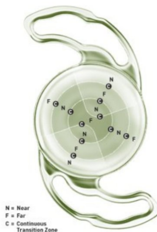
Figure 2.1.8: Optical design of the Precizon Presbyopic MIOL (Source: [41]).
