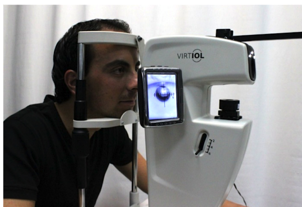
Figure 4.0.2: Image of VirtIOL while the patient is observing a vision test through the inserted MIOL.
