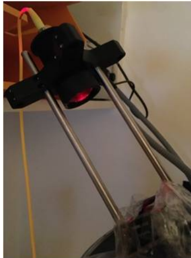
Figure A.2.5: Image of the new illumination system composed by the optical fiber of the laser and the achromatic doublet.
