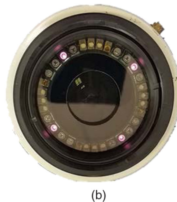
Fig. 2 LEDs included in the ring of the multispectral system: (a) spectral emission and (b) front picture of the ring.
