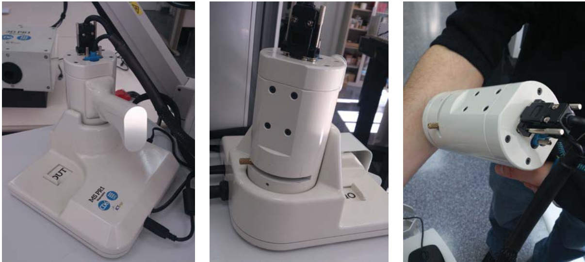
Figure 1: Different views of the handheld hyperspectral system.
