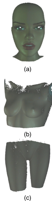
Figure 6. 3D cloud of points with RGB colour superimposed. (a) the face (b) the torso and (c) the upper part of the legs of a female mannequin.
