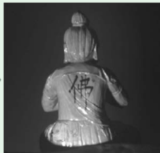
▲ Observation by IR light (C10633-13) The letter under lacquer is clearly visible.
