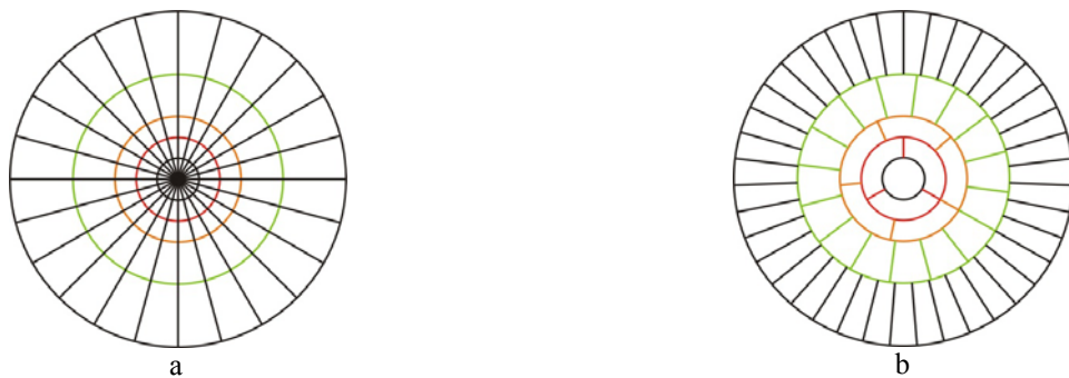
Figure 1: Example of segmentation methods. Segmentation method based on concentric division a) Geometric criteria: equiangular division b) energetic criteria :segments of equal area based on golden ratio
