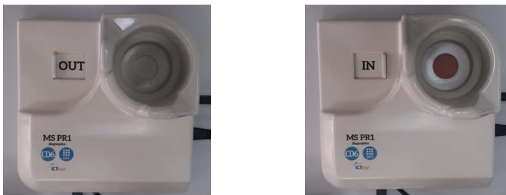
Figure 2: View of the base of the handheld hyperspectral system with the calibrated sample in the “out” and “in” positions, respectively.
