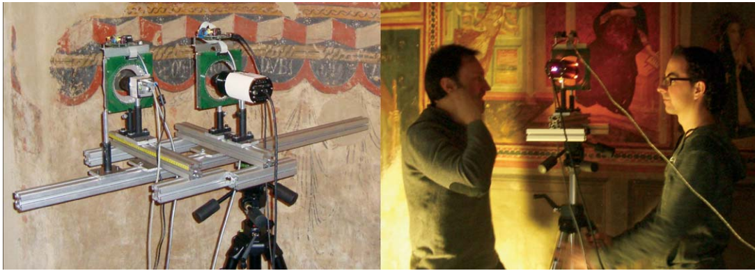
Fig. 1. Experimental setup of the portable multispectral system.
