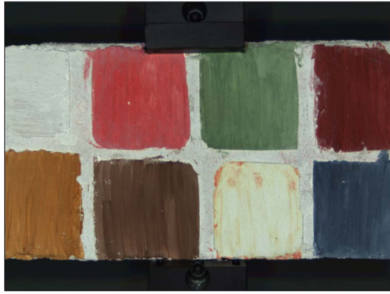
Fig. 8. Palette of pigments built emulating the fresco technique applied in wall paintings.
