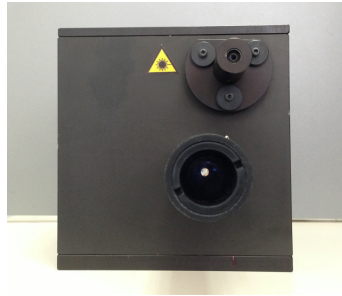
Figure 1. Front view of the prototype of lidar setup. The upper optical group illuminates the scene using a diverging optics. The lower one is used to capture the back reflected light onto the optical scanning system.
