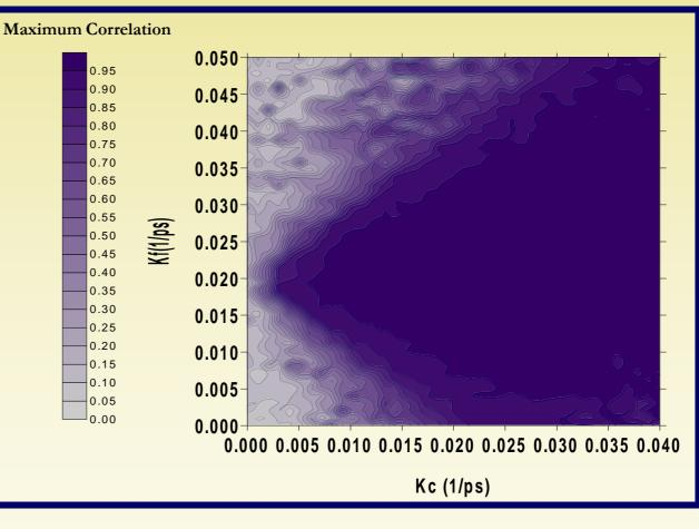
•Maximum of correlation function as a function of the coupling constant (Kc) and feedback rate (Kf) of LD-1 (feedback strength of LD-2 fixed at 20ns<sup>-1</sup>)
