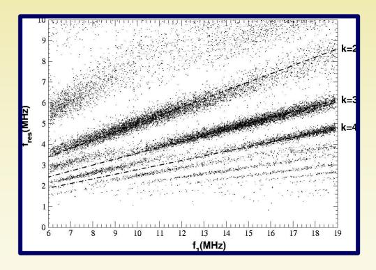
•Numerically determined response frequency between dropouts  $f_{res}$  as a function of  $f_1$
