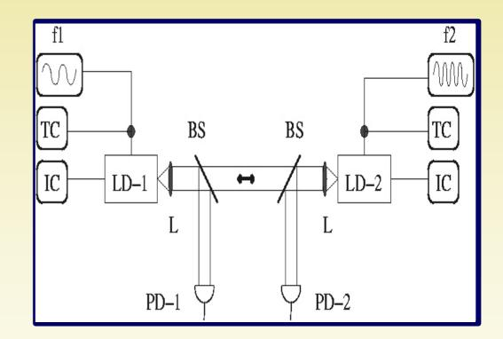
•When both lasers are independently modulated with two frequencies as  $f_1 = kf_0$  and  $f_2 = (k+1)f_0$ , coupling induces entrainment to a frequency not present at the input of any of the two lasers
