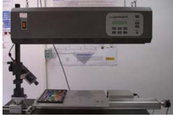
Figure 1. Hyperspectral system (camera, spectrograph and lens), illumination system (overhead luminaire) and linear scanning moving system.
