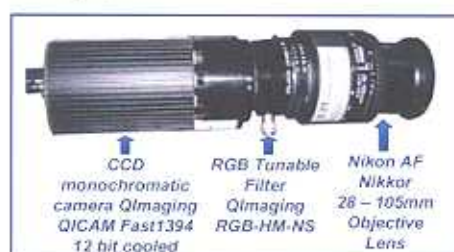
Fig. 2. Colorimetric configuration of the imaging system based on a 12 bits cooled monochromatic CCD camera.
