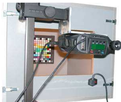
Figure 3. CCDC chart placed inside the light booth used in the experimental set-up and the tele-spectra-colorimeter used as reference instrument.
