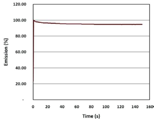
Figure 2. Curve of temporal stabilization of LED emission
