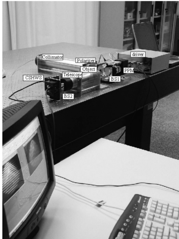
Figure 1. AO system constructed to test commercial lenses with complex shapes.
