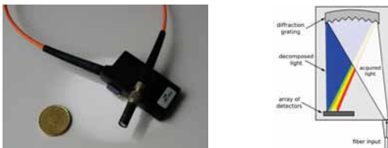
Fig. 3. Example of a miniature hyperspectral CMOS-array spectrometer designed for oceanographic monitoring purposes and its interior view (Pons et al., 2007). The concave grating splits the light collected through the input fiber and images each component in one detector in the array.
