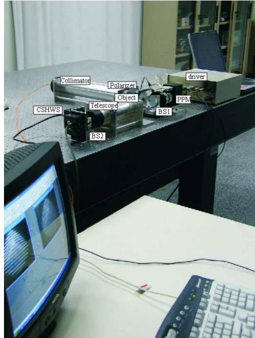
Fig. 1: Active null-test of complex-shaped optical objects, which is applied to personalized progressive addition lenses.
