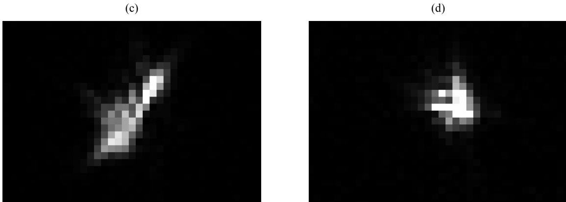
Fig.4-1.a) Image of the source plane before BFL adjustment; b) Image of source plane after BFL adjustment; c) Central PSF before BFL adjustment; d) Central PSF after BFL adjustment
