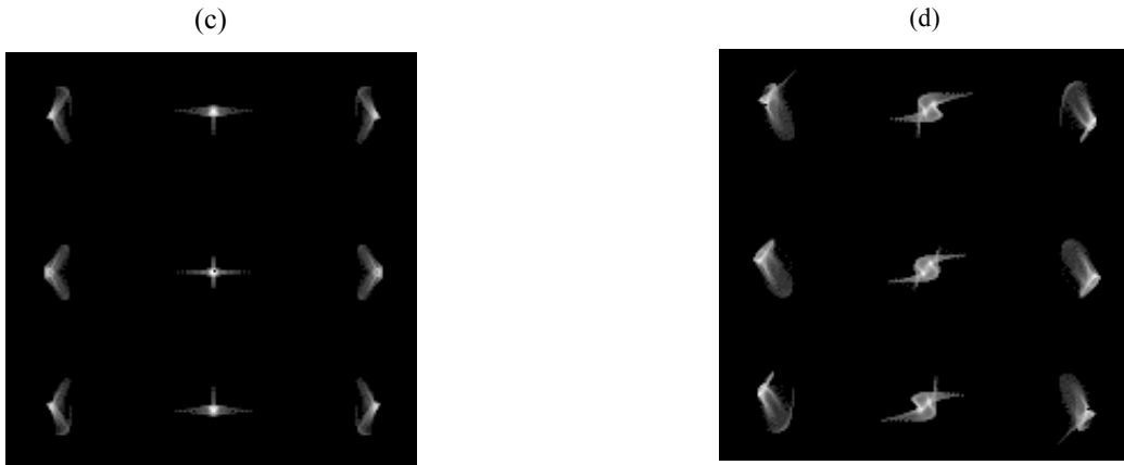
Fig.2-5. a) PSF map of an anastigmatic optical system. b) Procedure for enlarged PSf representation ; c) Perfectly aligned anastigmat; d) Axis of cylindrical lens tilted by 0.5^\circ
