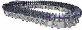
Bobinas toroidales (Iberdrola, Elytt)
