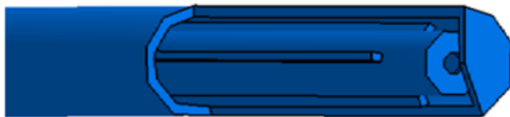
Coaxial, self-cooled irradiation end based on ITER NAS. Y. Lee, et al., Fusion Engineering and Design 89 (2014) 1894.
