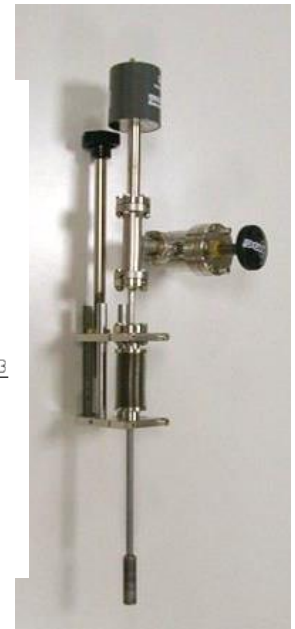
Coated membrane capsules (Pd on vacuum side) under development
