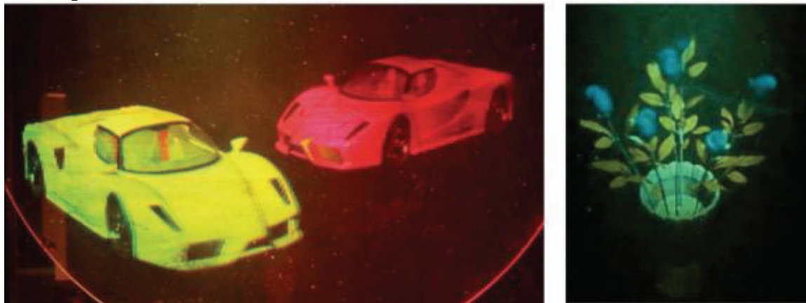
FIGURE 10.3: Pictures of colored holograms. (left) Hologram of two model cars recorded. (right) Hologram of a vase and flowers. SOURCE: Reprinted, with permission, from Blanche P.-A., A. Bablumian, R. Voorakaranam, C. Christenson, W. Lin, T. Gu, D. Flores, P. Wang, W.-Y. Hsieh, M. Kathaperumal, B. Rachwal, O. Siddiqui, J. Thomas, R. A. Norwood, M. Yamamoto, N. Peyghambarian. 2010. Holographic three-dimensional telepresence using large-area photorefractive polymer. Nature 468:80–83.
