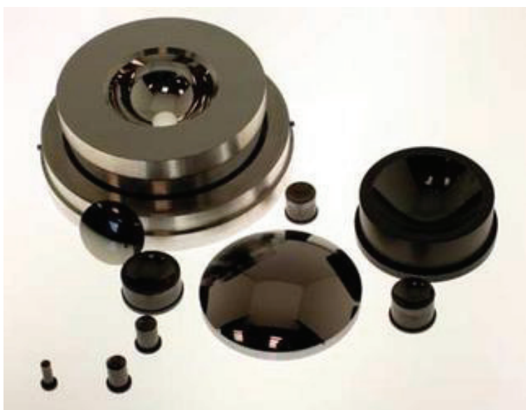
FIGURE C.10 Generic molding inserts and molded asphere lenses. SOURCE: Courtesy of Rochester Precision Optics.
