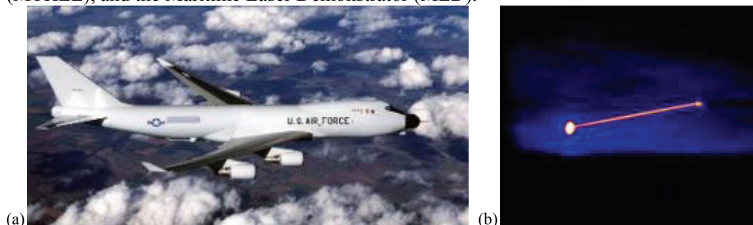
FIGURE 4.1 Airborne Laser Test Bed (ALTB). (a) The ALTB is a platform for the Department of Defense's directed energy research program. Two solid state lasers and a megawatt-class Chemical Oxygen Iodine Laser (COIL) are housed aboard a modified Boeing 747-400 Freighter. (b) An infrared image of the Missile Defense Agency's Airborne Laser Test Bed (at right in the image) destroying a threat representative short-range ballistic missile (at left in the image). SOURCE: Images available from the Missile Defense Agency, http://www.mda.mil/news/gallery_altb.html . Accessed on November 30, 2011.
