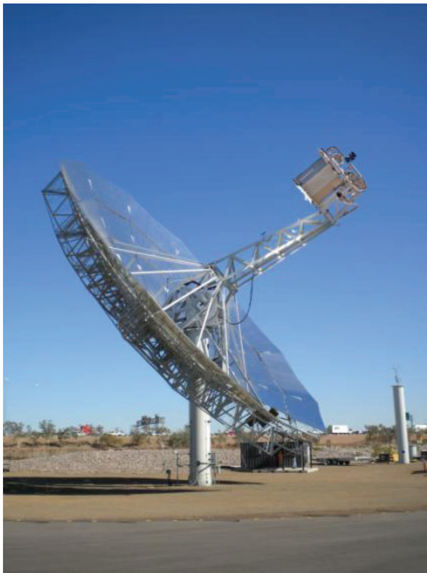
FIGURE 5.12 A dish solar thermal power generation module test unit in Phoenix, Arizona. The dish is approximately 75 feet in diameter. SOURCE: Courtesy of Southwest Solar Technologies.
