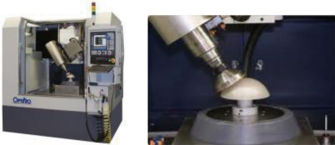
FIGURE C.8 (left) A commercially available 5-Axis Computer Numerically Controlled grinder. (right) a close up image of the grinding head. SOURCE: Courtesy of Optipro.
