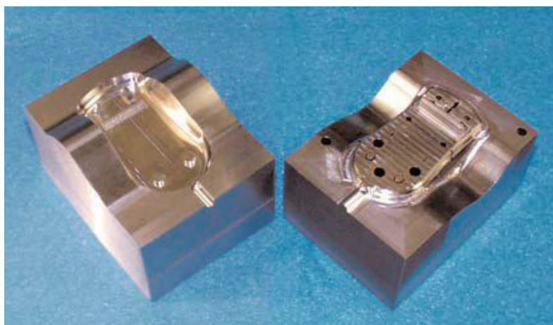
FIGURE 7.16: H13 tooling created with LENS™ process. SOURCE: Courtesy of Sandia National Laboratories.
