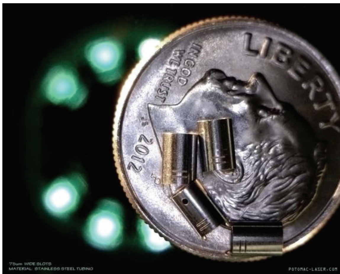
FIGURE 7.10: Slots cut into stainless steel are 75 \mu\text{m} wide. It should be pointed out that lasers are going to be needed in the future not only for machining but for interferometry for precision manufacturing. Laser interferometry is already being used in IC manufacturing for controlling etching and deposition on a nanometer scale and is going to be even more important in future high-resolution three-dimensional additive manufacturing. SOURCE: Courtesy of Potomac Photonics
