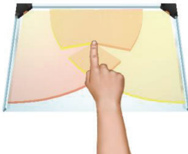
FIGURE C.24 Optical sensors in the upper corners of the array detecting touch. SOURCE: NextWindow. 2012. Optical Touch Overview. Available at http://www.nextwindow.com/optical/ . Accessed on July 31, 2012. Reprinted with permission.
